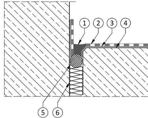
1. Filling of the expansion joint - NEXLER EPOLIS EP 603 Poziom
