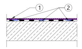
1. Renovation layers - NEXLER Izofol Roof
