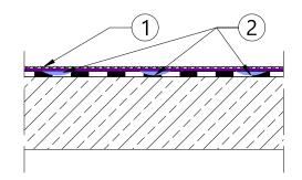
1. Renovation layers - NEXLER Izofol Roof
