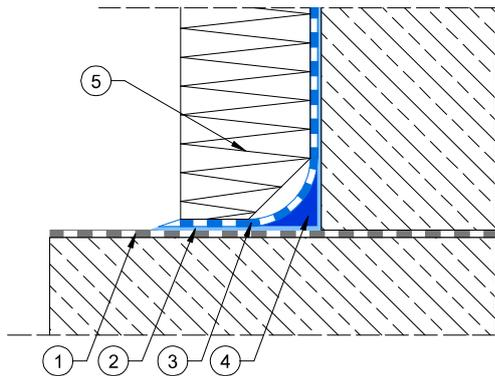
1. Horizontal insulation made of bituminous felt
